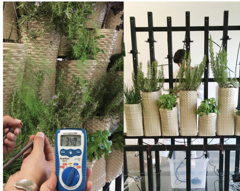
Figure 9 Voltage energy readings for one of the Green Leafs and the substructure of the supporting structural, irrigation and electrical systems
